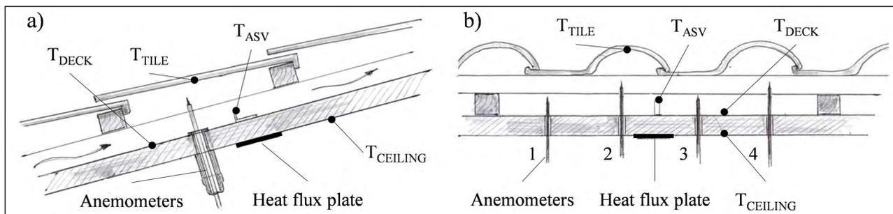
Figure 4 The monitoring section with sensors. a) Longitudinal section b) Cross section.
