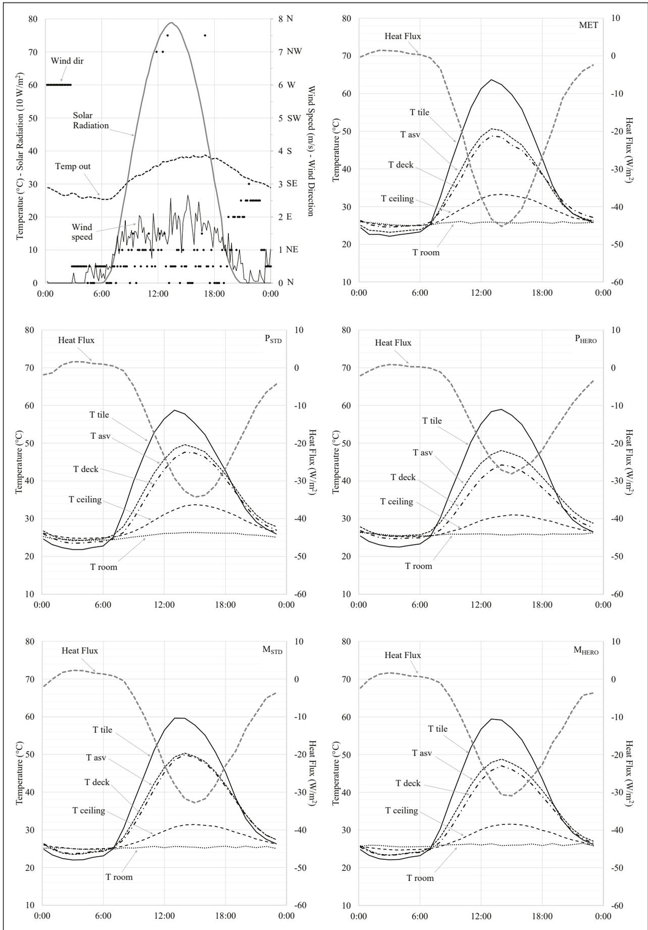
**Figure 5** Daily thermal behaviour of the ventilated roofs and local weather conditions.
