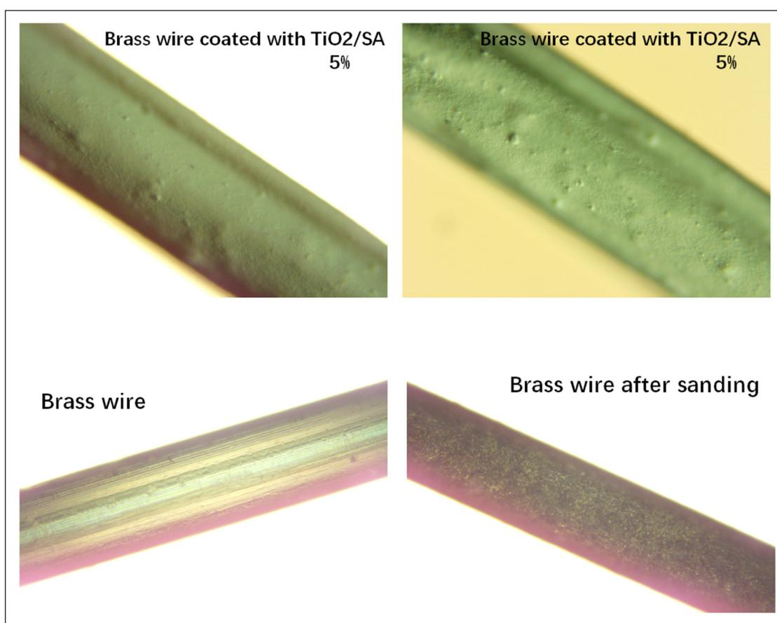
**Figure 8** Microstructure of the brass wire with and without coating.
