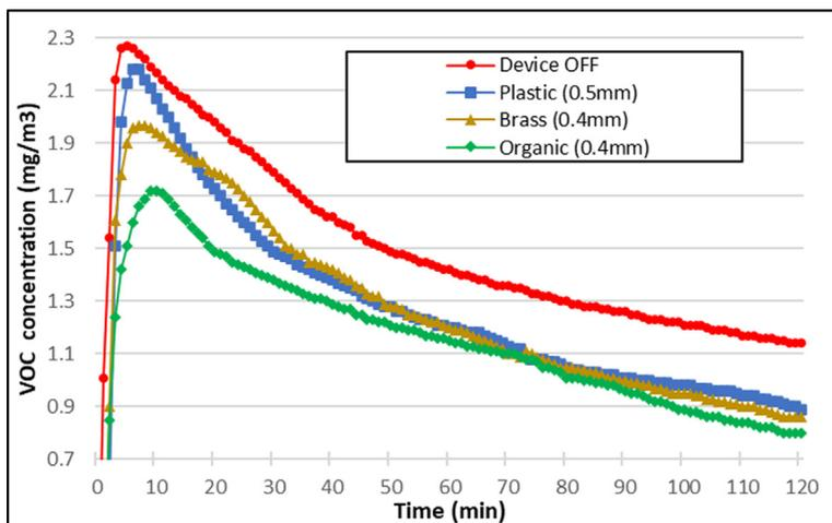
**Figure 16** Monitoring results of VOC concentration.
