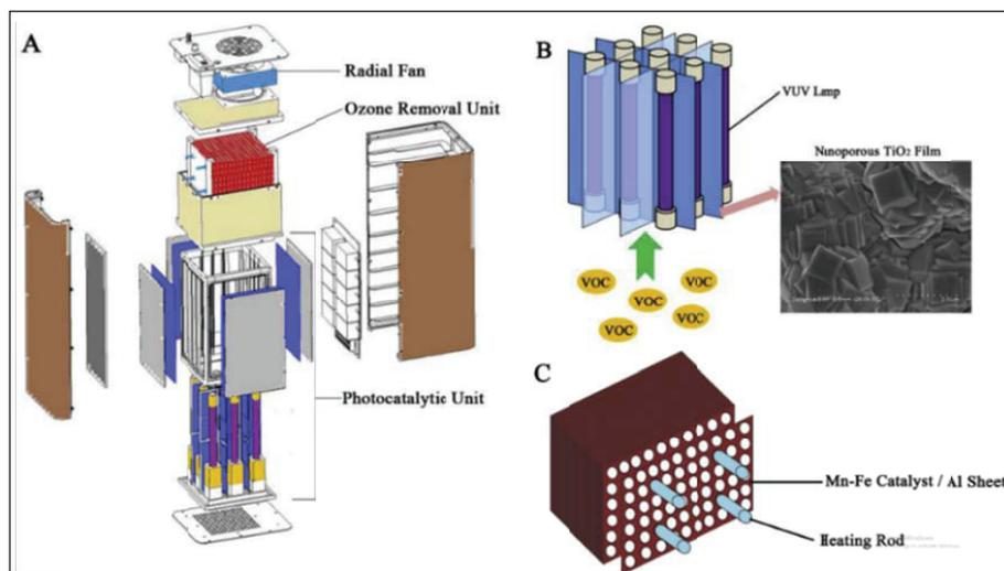
**Figure 1** Diagram of the VUV-PCO air purifier (A), the photocatalytic unit (B) and the ozone removal unit (C). (Xu et al, 2018).
