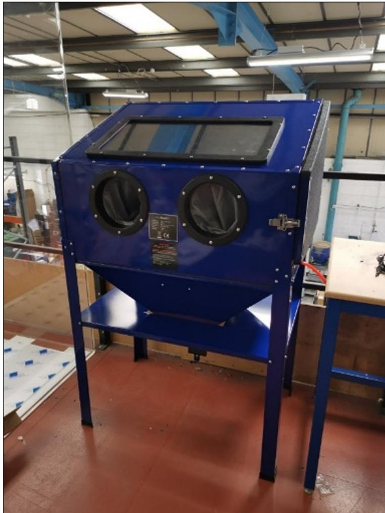
**Figure 3** MAXBLAST Heavy duty sand blasting chamber 220 L.
