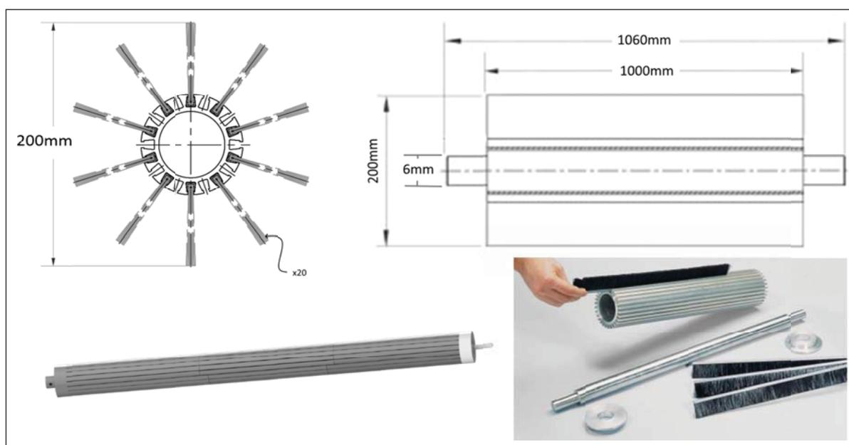
**Figure 9** Dimensions and design of the hub.
