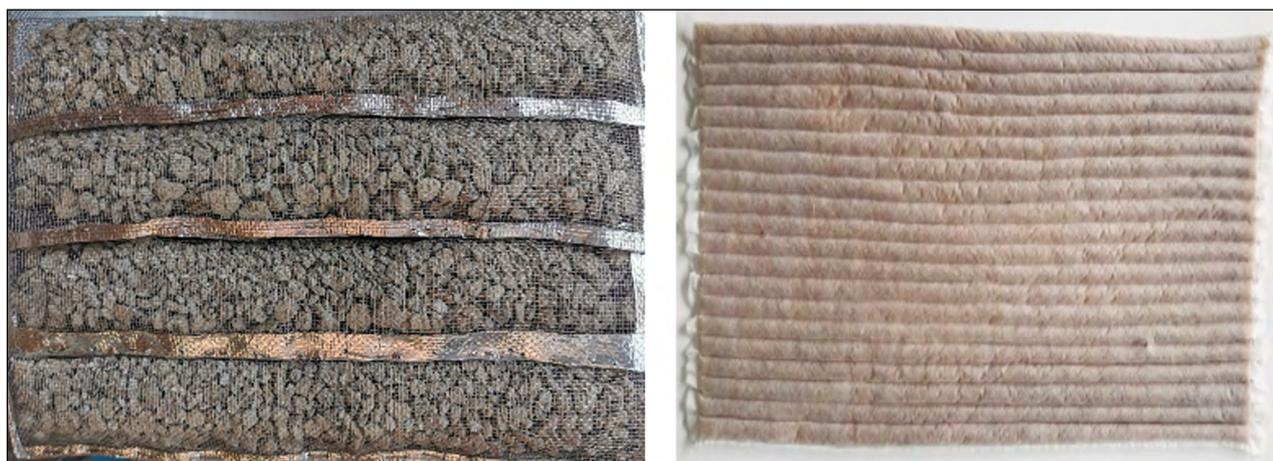
**Figure 1** ChainStore sheets filled with adsorbent heat storage materials.
