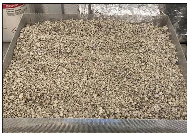
**Figure 4** Dried vermiculite based  $\text{MgSO}_4$ - $\text{CaCl}_2$  composite.
