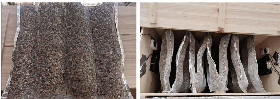
**Figure 8** ChainStore sheets with vermiculite-based composite.
