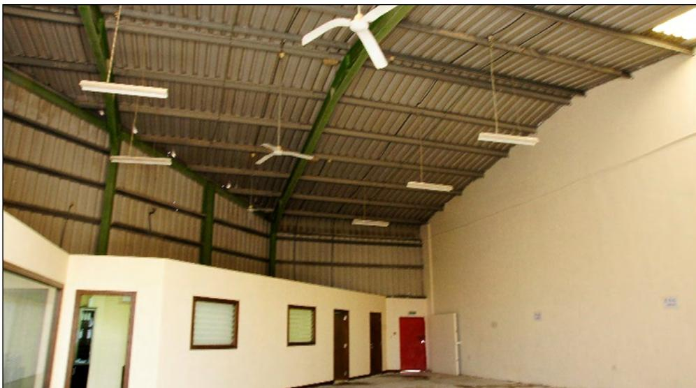
**Figure 4** Mixed conditioned space. The offices at the bottom of the picture are cooled; the remainder of the interior is not (by author).
