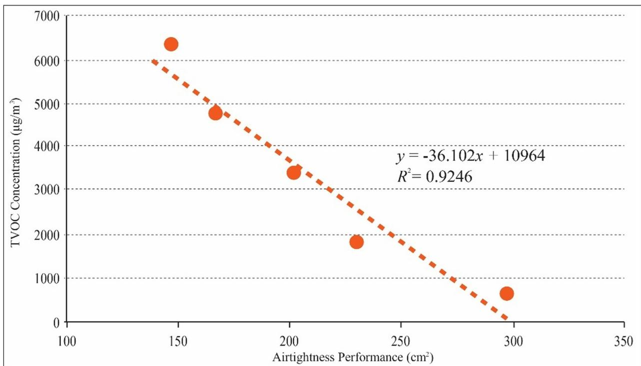
Figure 11 Comparative Analysis of Airtightness Performance and TVOC.
