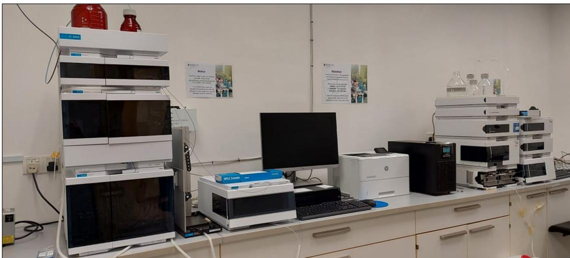
**Figure 1** High-Performance Liquid Chromatography.
