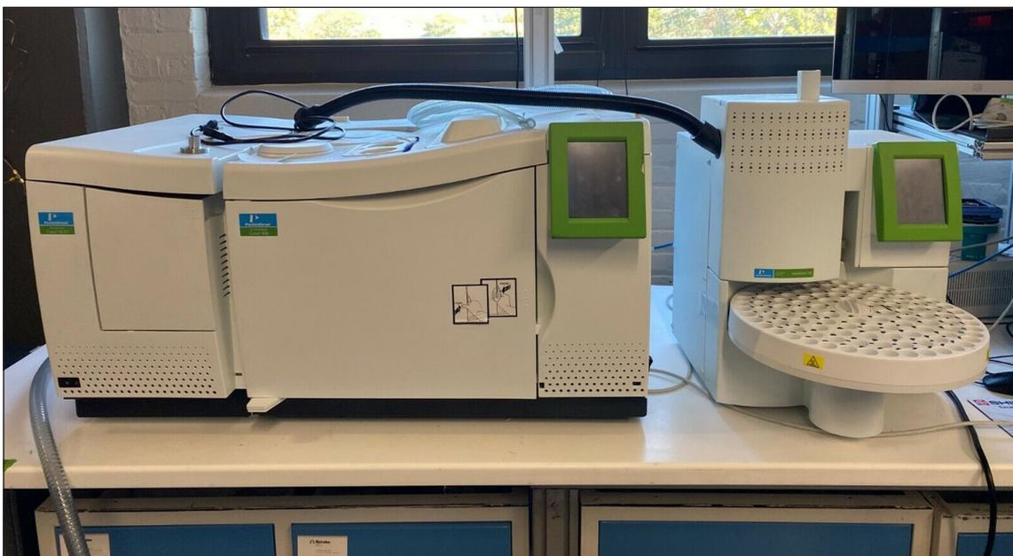
**Figure 2** Gas Chromatography-Mass Spectrometry.
