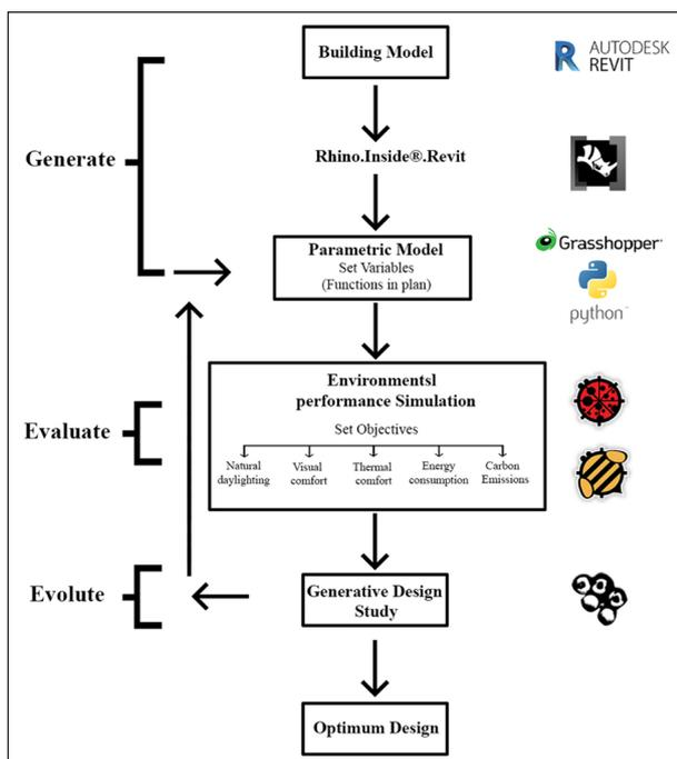
Figure 4 Generative design procedure.
