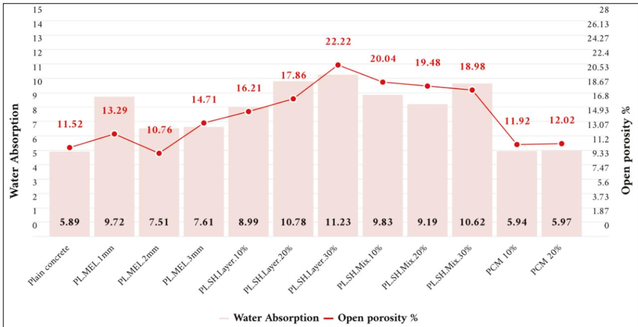
**Figure 5** Relationship of water absorption with porosity.
