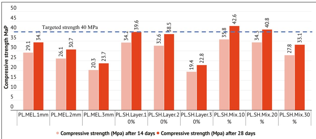
Figure 7 Compressive strength and load results.
