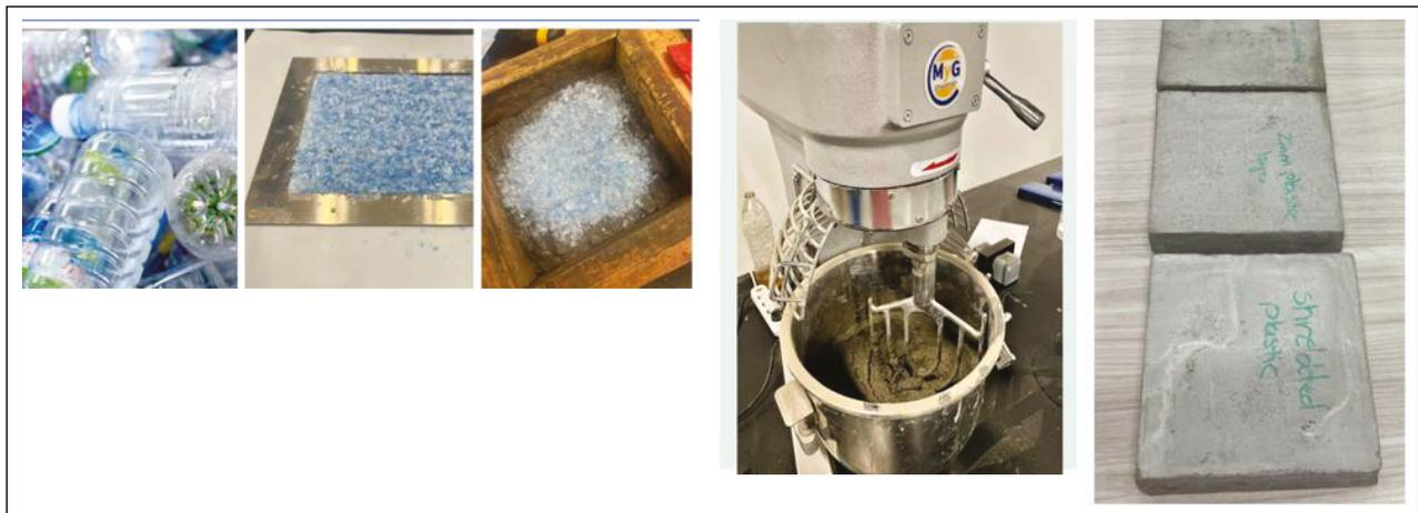
**Figure 2** Images of the shredded waste plastic and combining them with concrete to have concrete samples with plastic.
