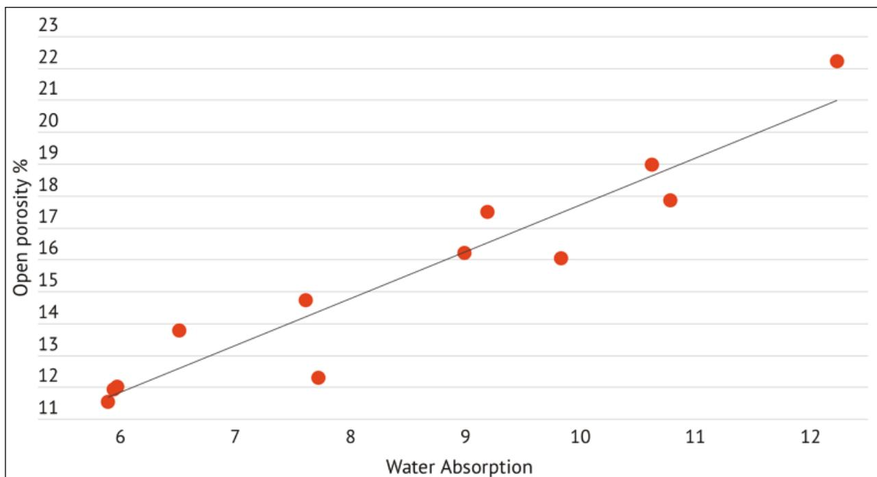
**Figure 6** The correlation between the porosity of concrete and its water absorbability.
