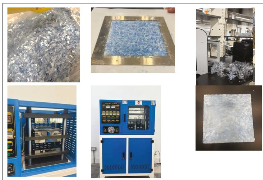
**Figure 1** Images of the shredded waste plastic before and after melting to convert to solid layer or use it as shredded layer.
