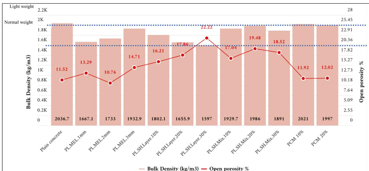
**Figure 4** Relationship of bulk density with porosity.
