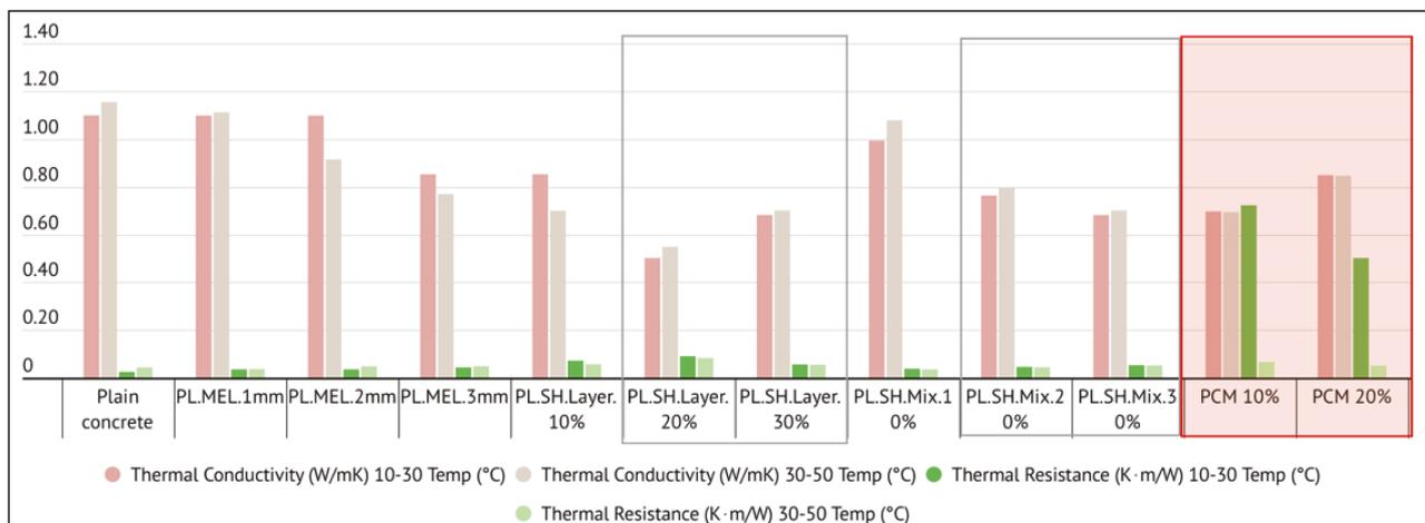
Figure 8 Thermal conductivity in two temperature range (10–30 C, 30–50 C).
