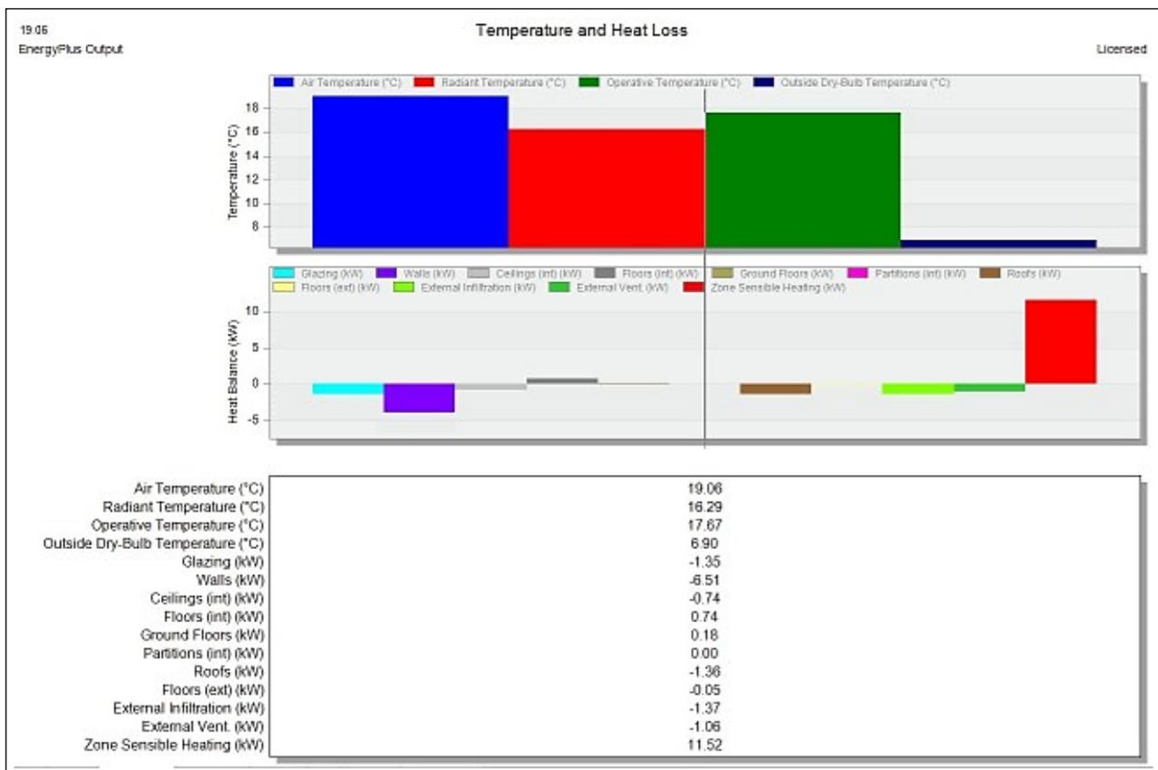
**Figure 13** Temperature and heat loss.
