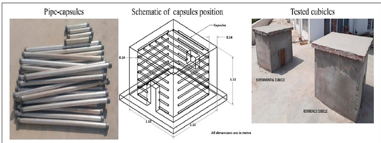
**Figure 4** The indicated installation procedures for pipe macro-encapsulated PCM (Al-Yasiri & Szabó, 2021).
