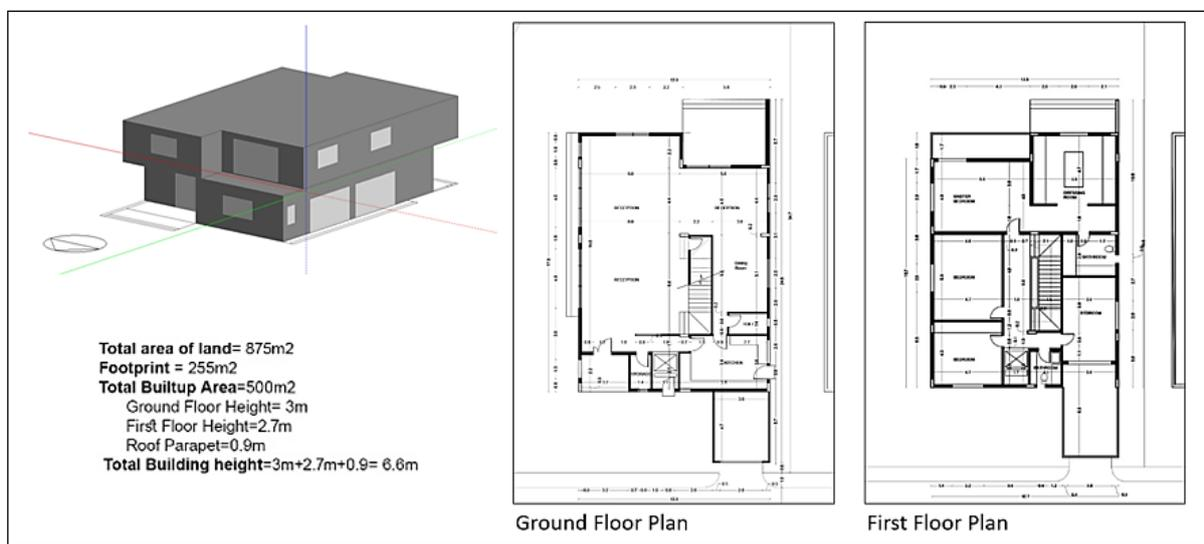
Figure 7 Architectural plans and Design Builder model of studied building.
