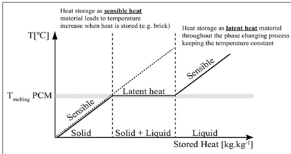
**Figure 1** Sensible heat and Latent heat storage for the case solid-liquid (Bhamare et al., 2017).
