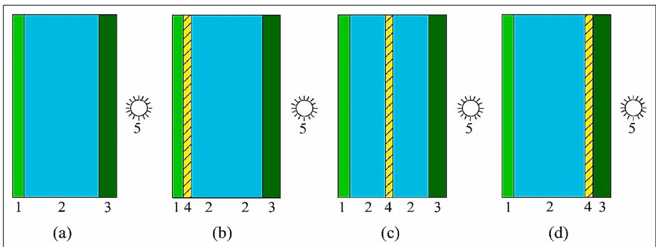
**Figure 5** Diagram illustrating the placements of the PCM layers that were studied: (a) ordinary wall; (b) PCM layer placed near the interior; (c) PCM layer positioned in the centre; and (d) PCM layer placed near the exterior.
