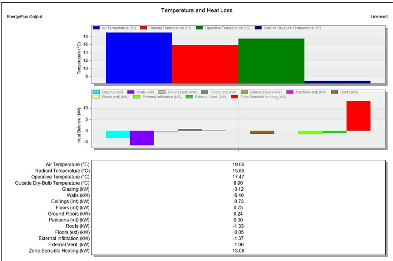
**Figure 10** Temperature and heat loss.
