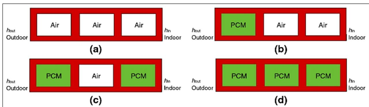
**Figure 3** Bricks with PCM integration models (Tunçbilek et al., 2020).
