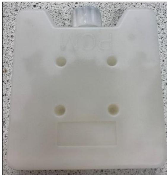
**Figure 3:** Thermal conductivity S23 sample panel.
