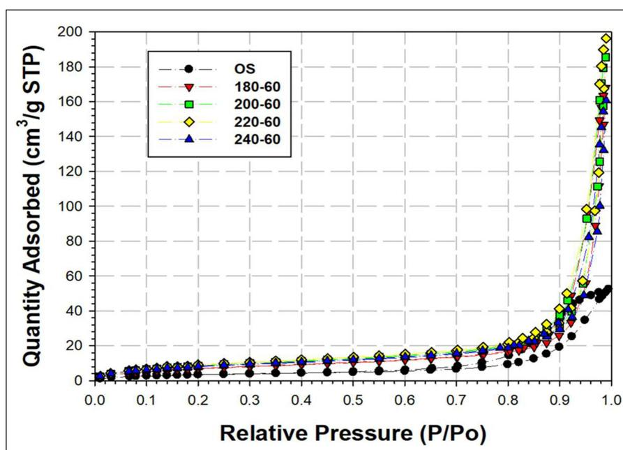
**Figure 7:** The adsorption isotherm of organic sludge (OS) and hydrochar under various HTC conditions ( $T = 180, 200, 220, 240\text{ }^\circ\text{C}$ ;  $t = 60\text{ min}$ ).
