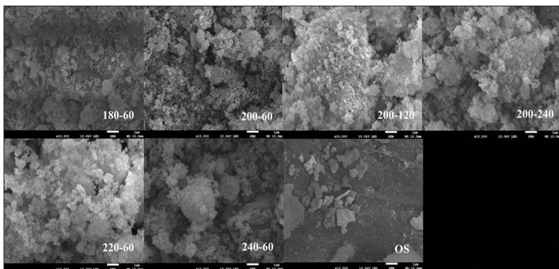
**Figure 4:** SEM images of organic sludge and hydrochar derived from different HTC conditions (OS: organic sludge; 180–60 represents hydrochar obtained from 180 °C, 60 min.).
