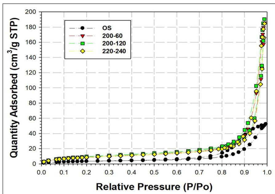
**Figure 8:** The adsorption isotherm of organic sludge (OS) and hydrochar under various HTC conditions (T = 200 °C; t = 60,120, 240 min).
