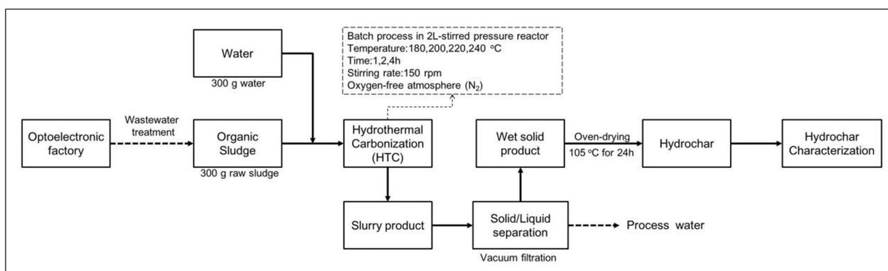
**Figure 1:** The schematic diagram of research process.
