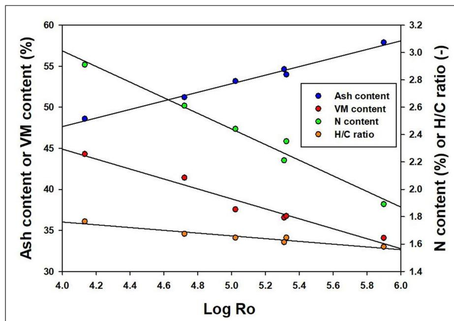
**Figure 3:** The relationship between hydrochar properties and HTC reaction severity (with ash content  $R^2 = 0.9882$ ; volatile matter  $R^2 = 0.9598$ ; N content  $R^2 = 0.9786$ ; and H/C ratio  $R^2 = 0.9317$ , respectively).
