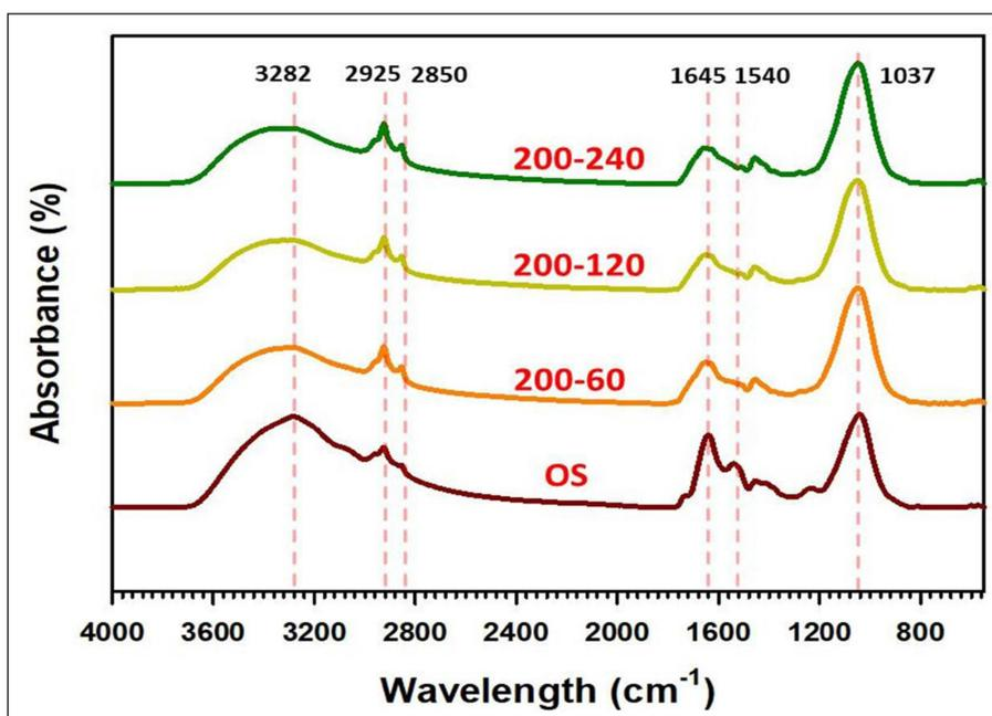
**Figure 6:** FT-IR spectra of organic sludge (OS) and hydrochar under various HTC conditions (T = 200 °C; t = 60,120,240 min).
