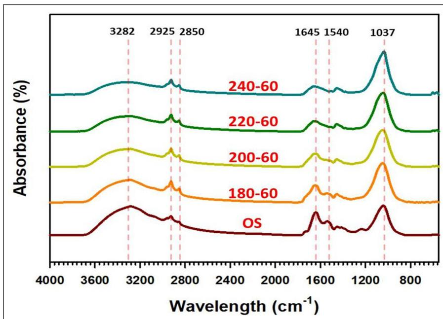
**Figure 5:** FT-IR spectra of organic sludge (OS) and hydrochar under various HTC conditions (T = 180,200,220,240 °C; t = 60 min).
