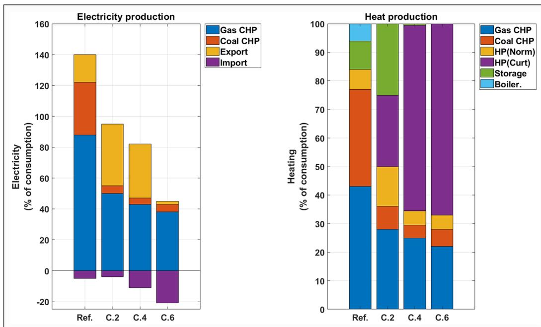
**Figure 5:** Electricity production and heat production of the power plants with different building energy savings, 1500 MW of heat pumps, and wind curtailment for Scenario 3 (cases 2, 4 and 6 in Table 6).
