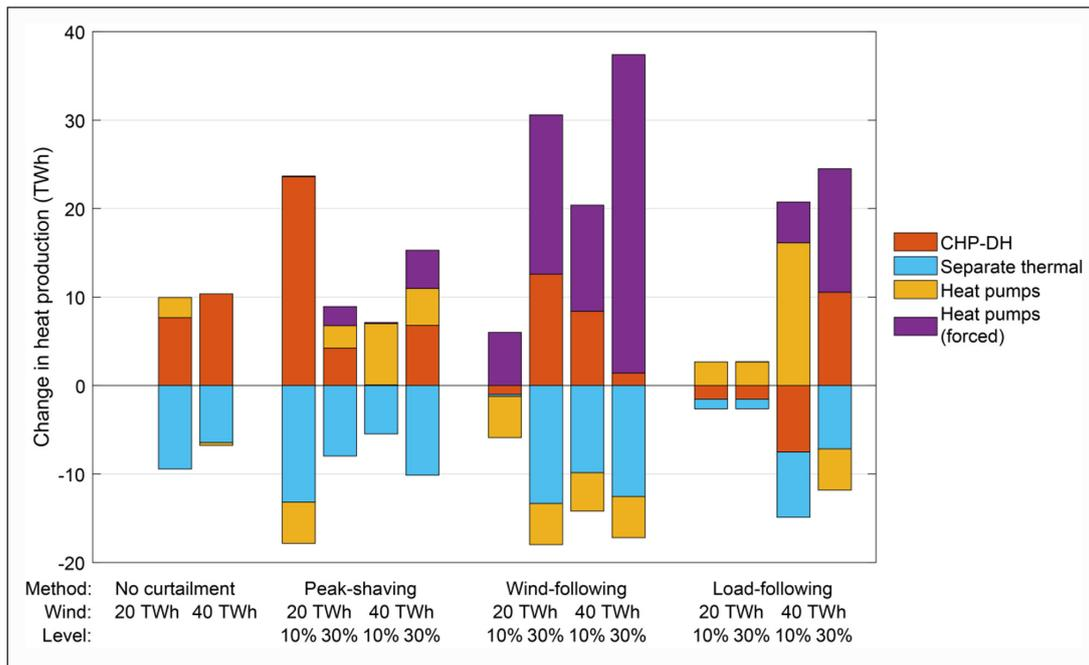
**Figure 2:** Change in the heat production compared to the national reference case (Finland 2013). “CHP-DH” refers to district heating CHP. Heat pump operation is divided into normal heat pump operation and “forced” heat pump operation using the curtailed wind power.
