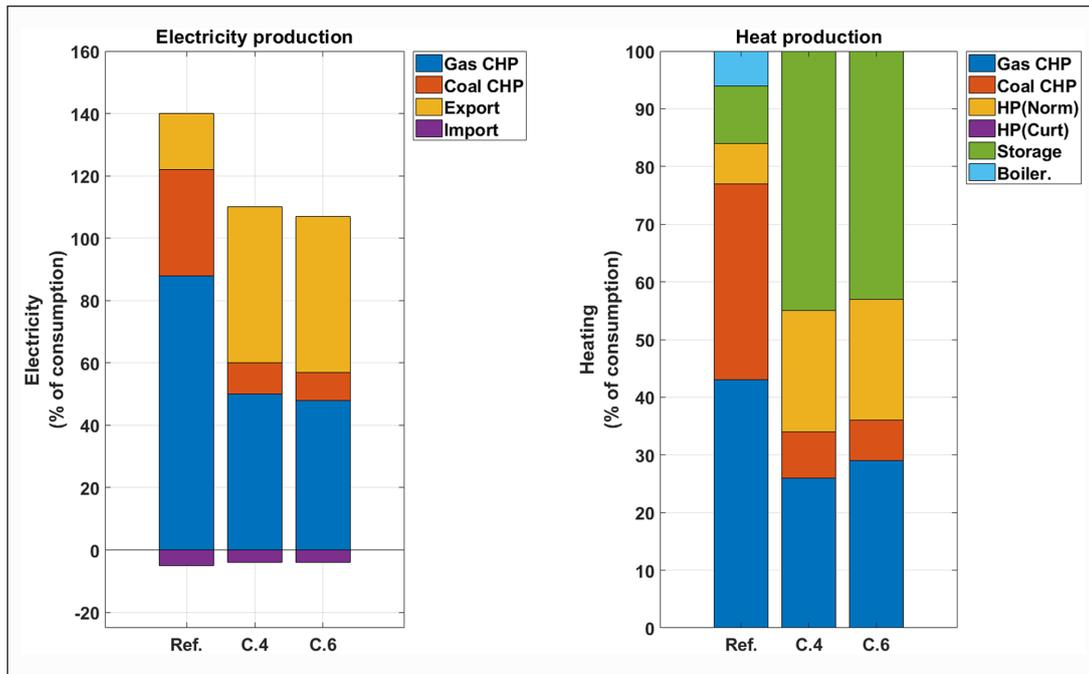
**Figure 4:** Electricity production and heat production of the power plants with different building energy saving levels and 1500 MW of heat pumps for Scenario 2 (cases 4 and 6 in Table 5).
