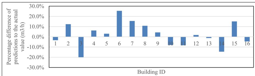
**Figure 11:** Percentage difference of predictions of  $Q_{50}$  to that measured by BD-M4.
