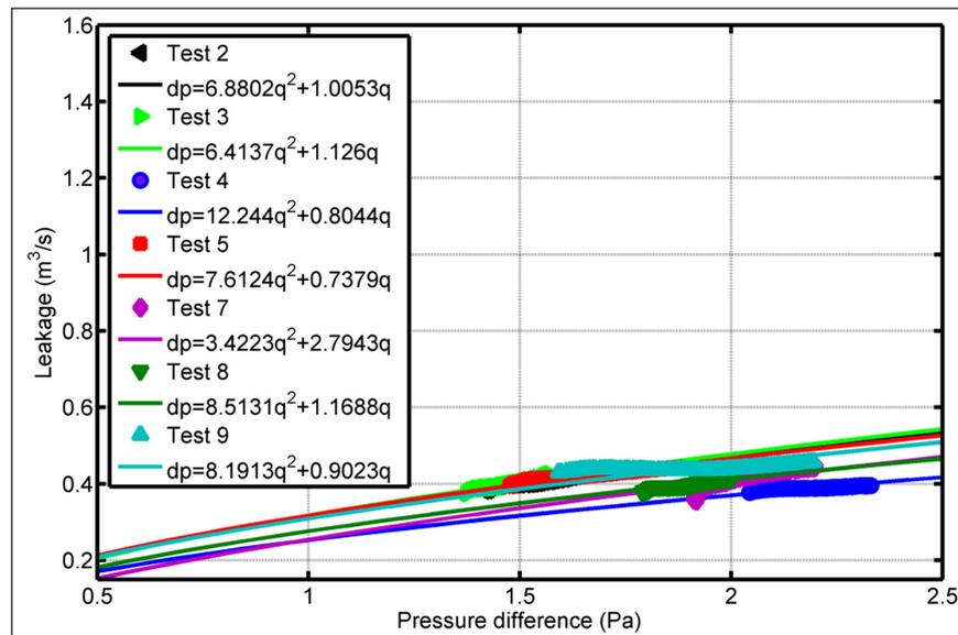
**Figure 16:** Leakage characteristic and power law fitting when vents were unsealed.
