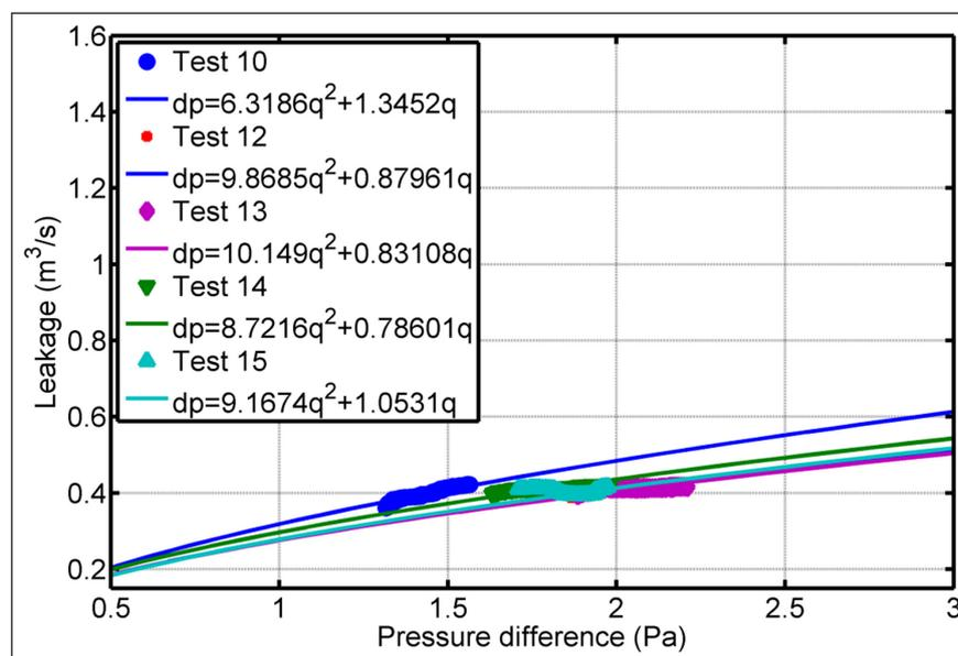
**Figure 17:** Leakage characteristic and power law fitting when vents were sealed.
