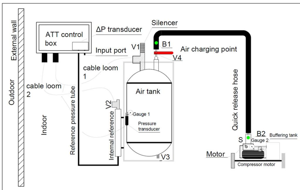
**Figure 7:** Schematic diagram and photo of the nozzle unit.
