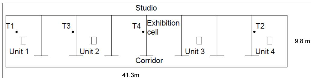
**Figure 13:** Floorplan of EEC Studio and locations of pistons/nozzles and internal pressure tappings (T1-T4).
