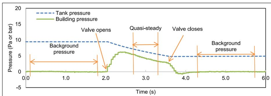
**Figure 3:** A typical pulse test by a unit with 60 l tank (tank pressure measured in bar, building pressure in Pa).
