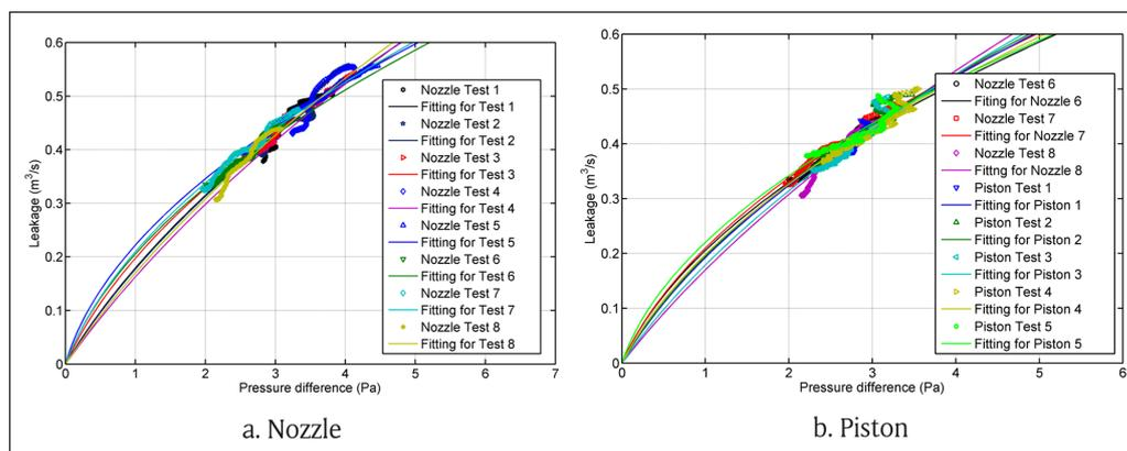
**Figure 14:** Leakage characteristic measured by piston and nozzle based pulse units.
