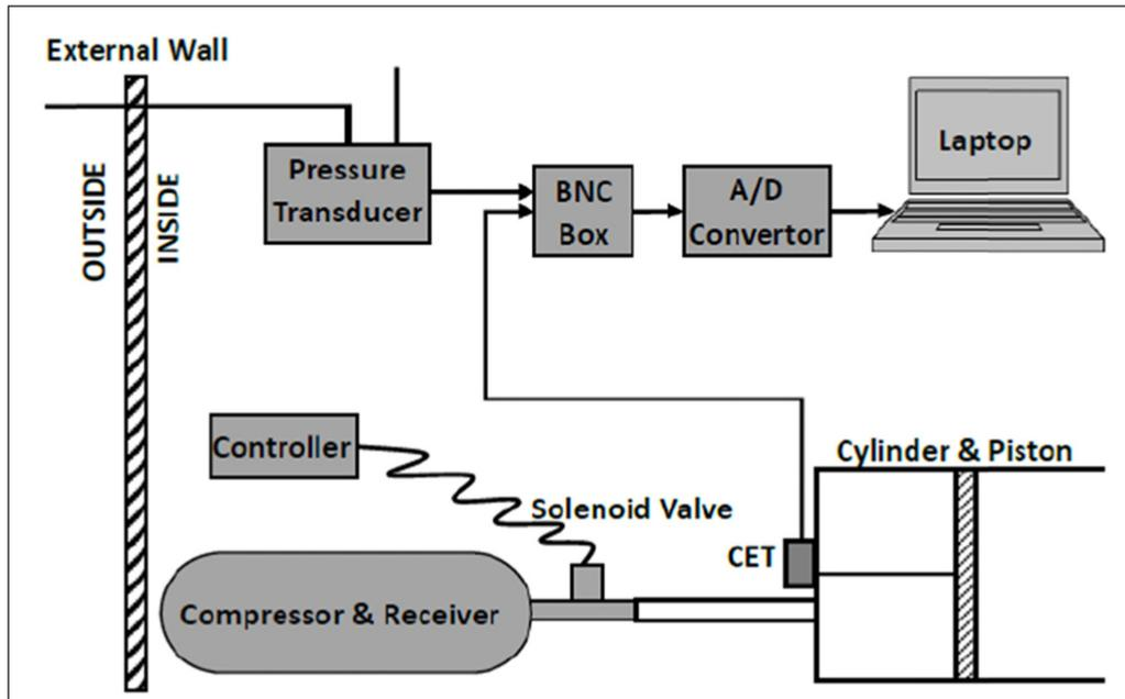
**Figure 6:** Schematic diagram of pulse technique using piston unit.
