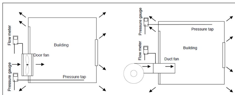
**Figure 1:** Steady state airtightness method (door fan and duct fan: in pressurisation).
