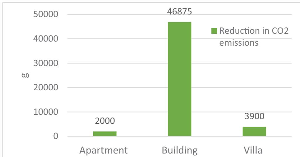
**Figure 11:** Reduction in CO<sub>2</sub> emissions by the use of PV panels for each property.
