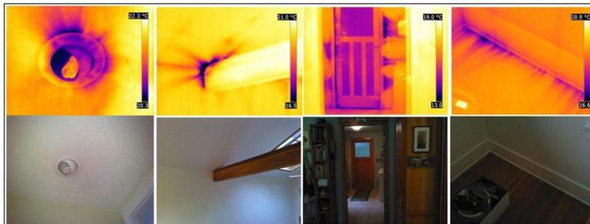
**Figure 3:** Thermal infrared images that show heat leakage from different parts of a house. Image taken from (Ahomecheck, 2018).
