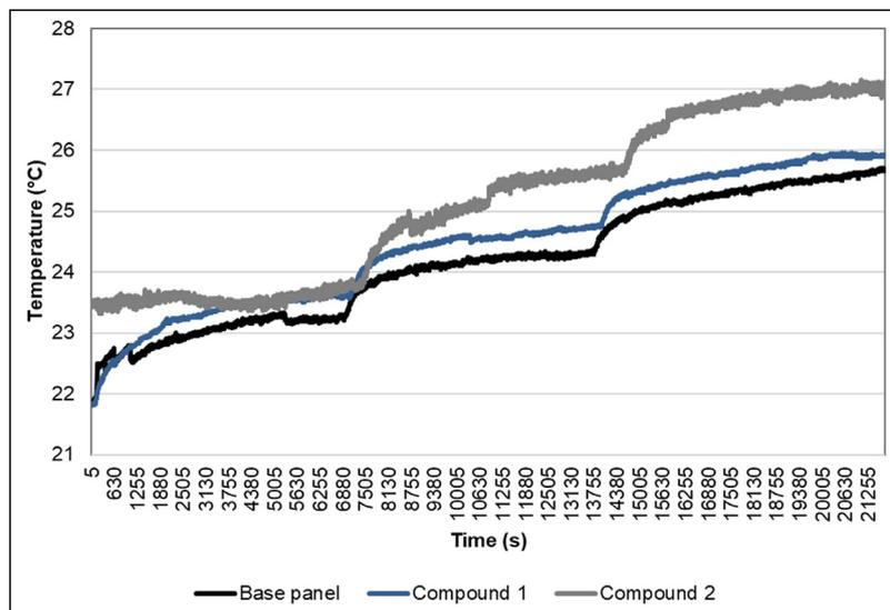
**Figure 7:** Test 2 – Blister panels comparison with 2 °C increments.
