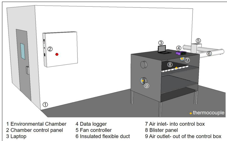
Figure 1: Schematic setup of the panel rig.
