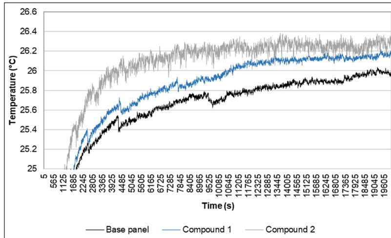
**Figure 6:** Test 1 – Blister panels comparison at 28 °C.
