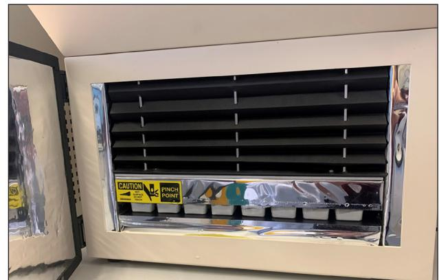
**Figure 5:** HFM-100 thermal conductive analysis of the blister panel.
