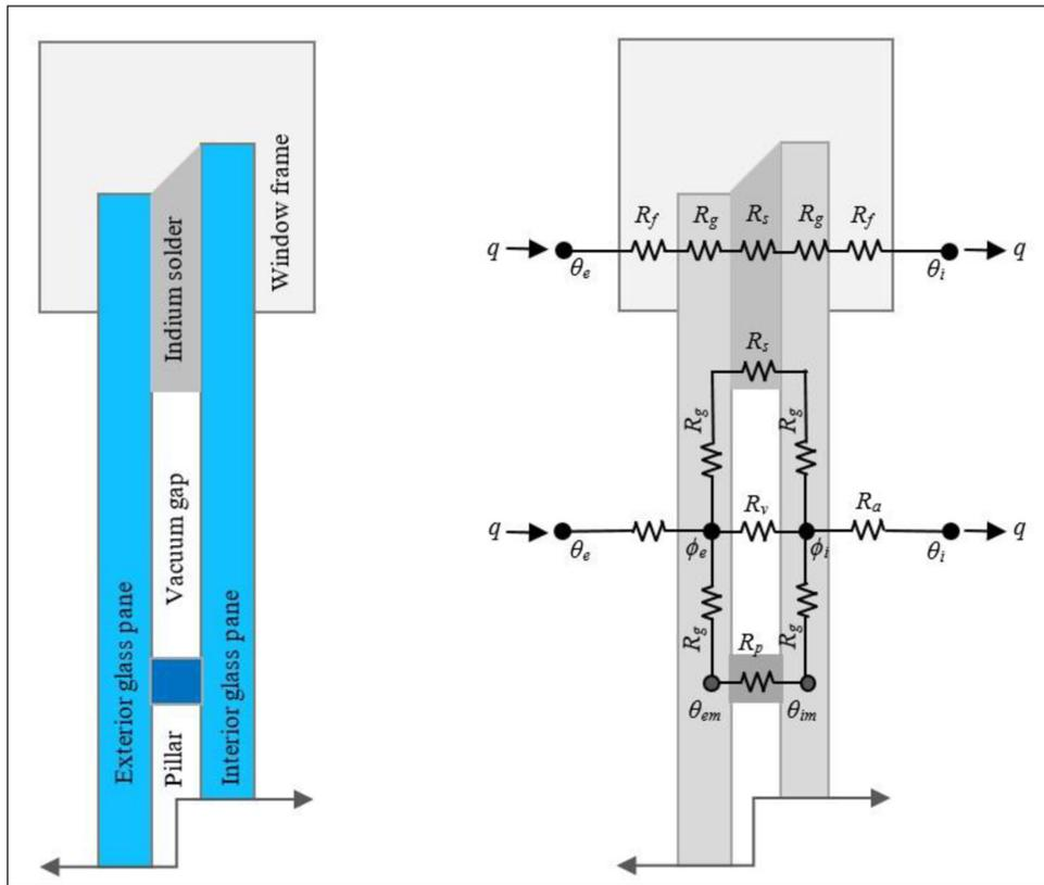
**Figure 2:** Layer composition and thermal circuit model for testing vacuum windows using the HFM method.
