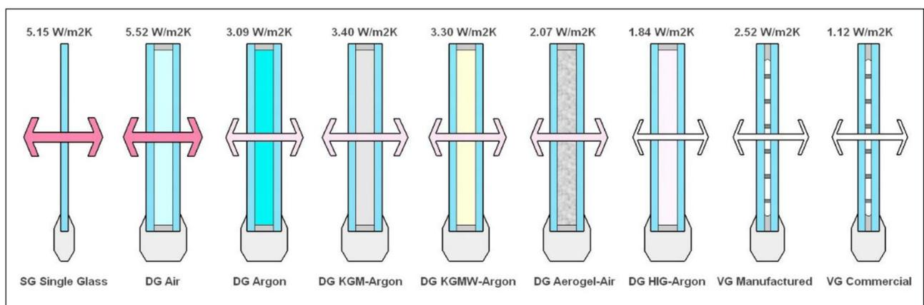
**Figure 10:** Thermal transmittance (U-value) of the nine novel window prototypes tested.
