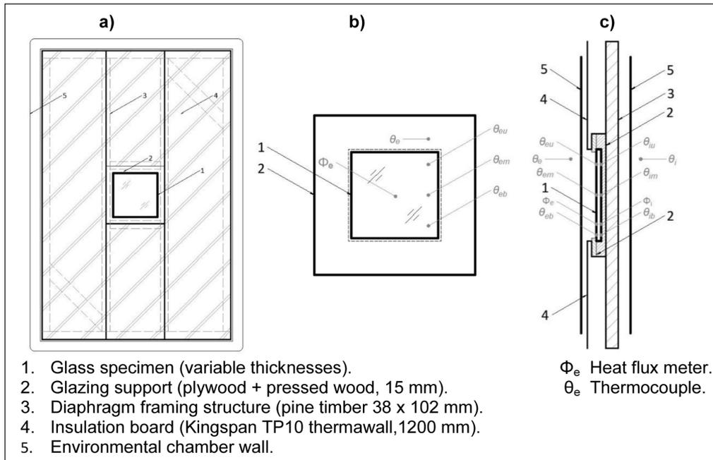
**Figure 4:** Details on the setup construction: **a)** environmental chamber testing plane, **b)** glazing support assembly, **c)** section of experimental wall.
