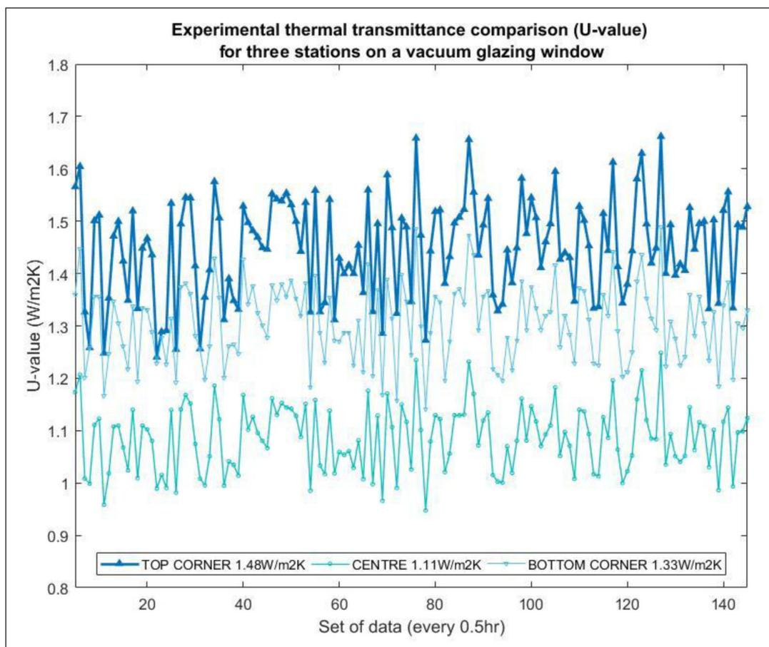
Figure 9: U-value comparison for the top, centre and bottom section of a commercial vacuum window.
