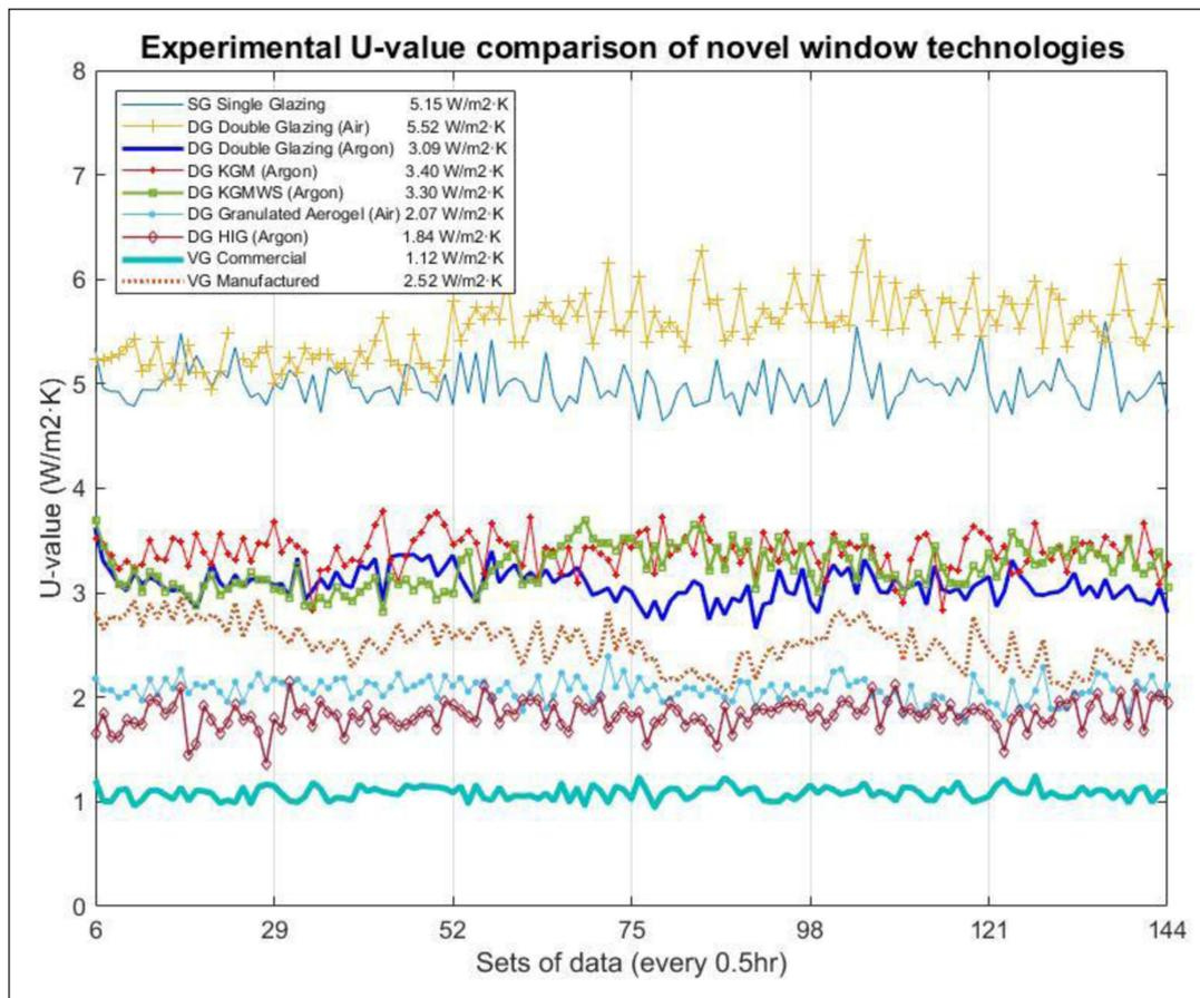
Figure 8: Thermal transmittance comparison of window samples over a 72-hours period.
