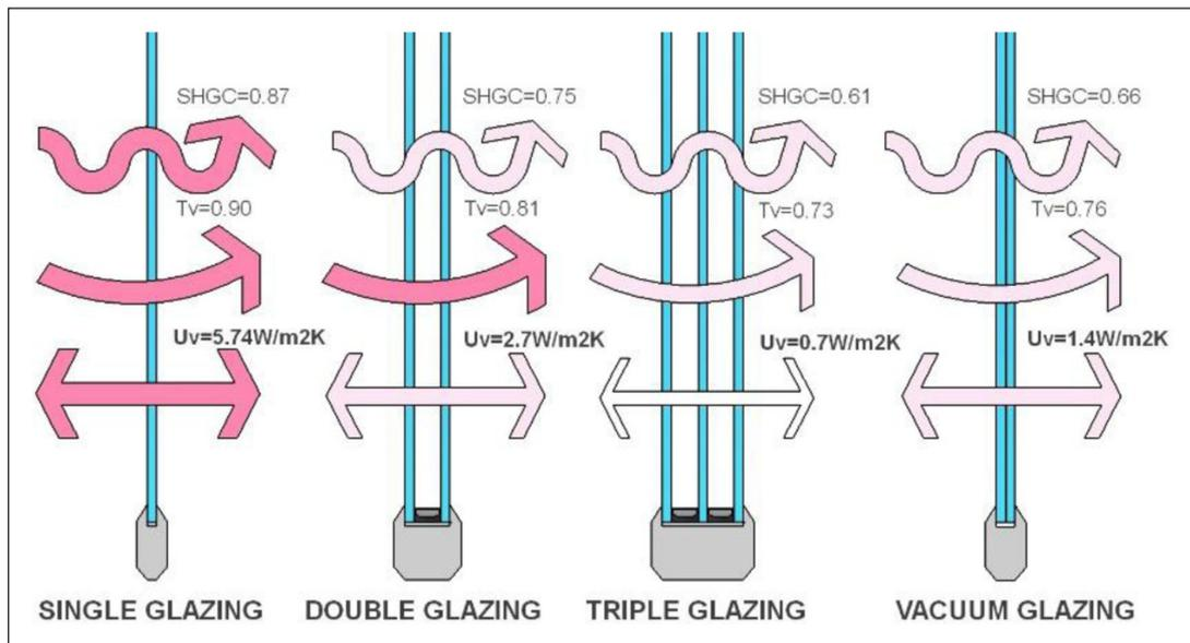
**Figure 1:** Thermal and optical properties of static windows (Aguilar-Santana, et al., 2020).
