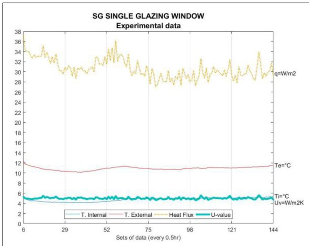
**Figure 6:** Experimental data of thermal transmittance for the single glazing window.
