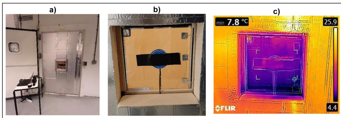
**Figure 5:** Experimental rig (a), manufactured vacuum glazing sample in test (b) and its infrared thermography (c).
